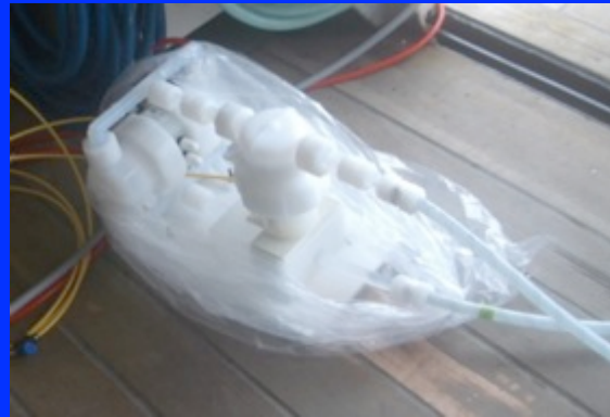
AstiPure PFD2 pump with AMC Pulsation Damper (Saint-Gobain)
