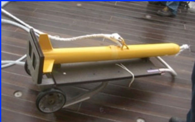
Epoxy-coated fish (10.2 cm \phi ×120 cm, 75 kg)
