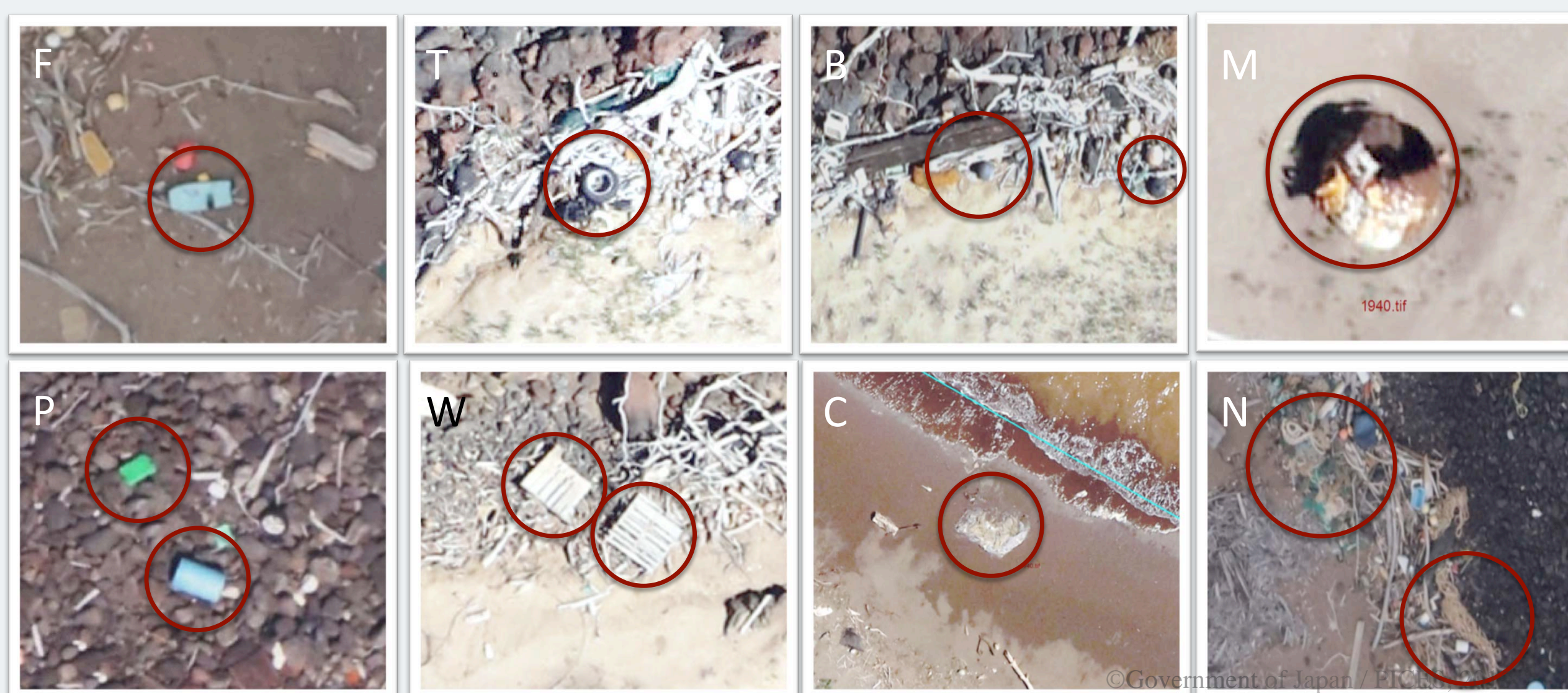
Figure 2. Examples of debris classifications from the aerial imagery: (F) foam, (T) tire, (B) buoys & floats, (M) metal, (P) plastics, (W) processed wood, (C) cloth, and (N) net & line. Not pictured: (V) vessels, (O) other or (U) unknown.
