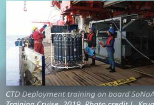
CTD Deployment training on board SoNoAT Training Cruise, 2019. Photo credit: L. Krug
