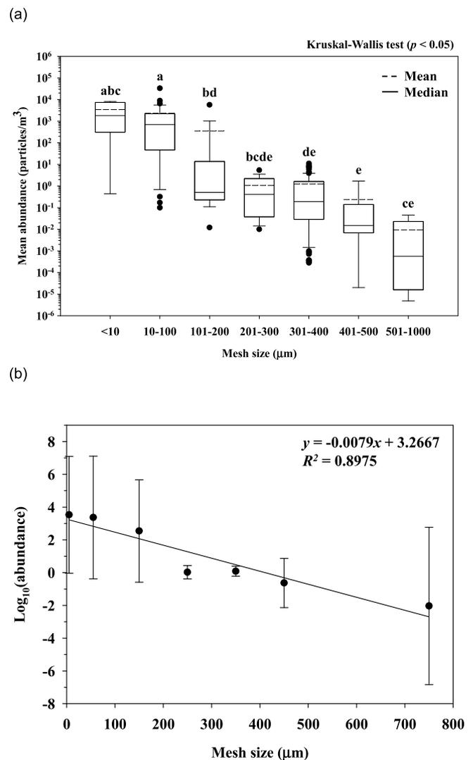
**Fig. 1.** Average abundance of (a) microplastics in seawater of the world ocean according to the minimum cut-off size range in sampling or analysis and (b) relationship between logarithmically transformed average abundance and the minimum cut-off size. Mean values with the same letter designation in boxplot (a) are not significantly different (Kruskal-Wallis test;  $p < 0.05$  and subsequent Mann-Whitney  $U$  test;  $p < 0.002$ ).
