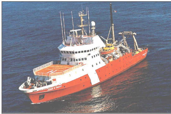
Fig. 2 The CGSS John P Tully, a 69 m research vessel operated by Fisheries and Oceans Canada to conduct oceanographic programs in the North Pacific.
