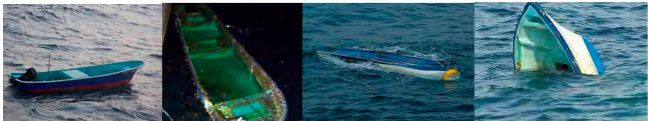
Fig. 7 Examples of JTMD boat orientation in water (from left to right): normal, upright but filled with water, upside down, and vertical. (Photographs courtesy of the Japan Coast Guard: http://www.kaiho.mlit.go.jp/info/kouhou/jisin/20110311miyagi/hyouryuu.htm )
