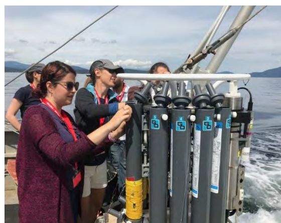
Preparing the CTD-rosette for water column sampling in Saanich Inlet.
