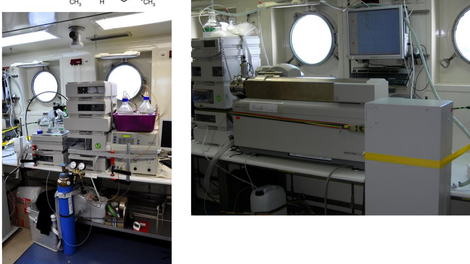
Analysis of marine toxins by liquid chromatography with fluorescence (LC-FD) or tandem mass spectrometry (LC-MS/MS)
