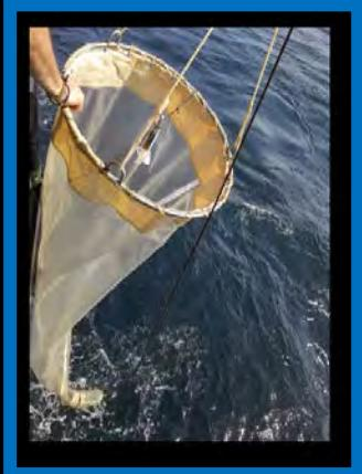
Conical net (333 µm)
