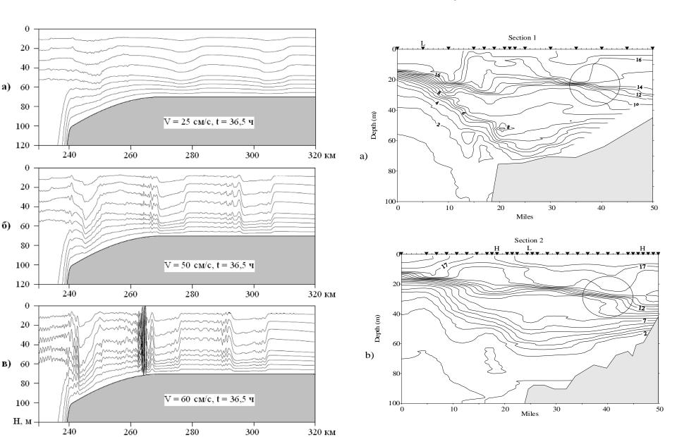
Internal waves transformation on the way from an open sea to a shore Measurements are made with the help of a towed line sensor
