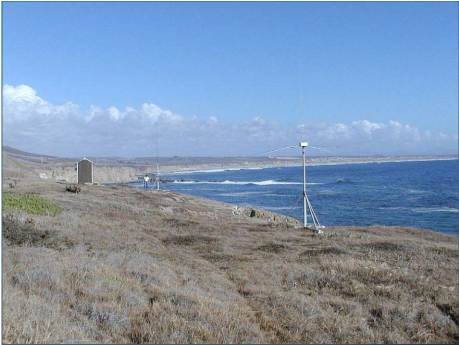
Typical CODAR deployment with transmit/receive antennae and electronics enclosure
