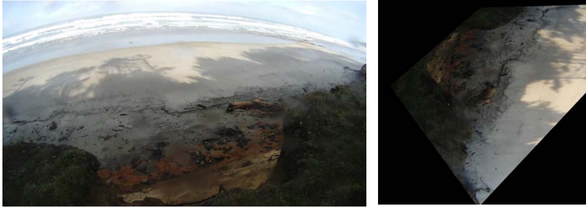
Fig. 3 Photo taken by the webcam at 1000EST on 4 April 2015 (a: left) and processed images by rotating the same photo onto the Cartesian coordinate with the projective transformation technique (b: right).
