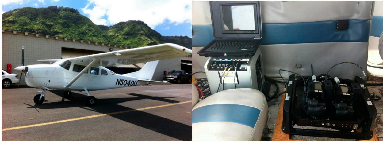
Fig. 1 RMH's Cessna 206 and IDM mapping system for image capture.
