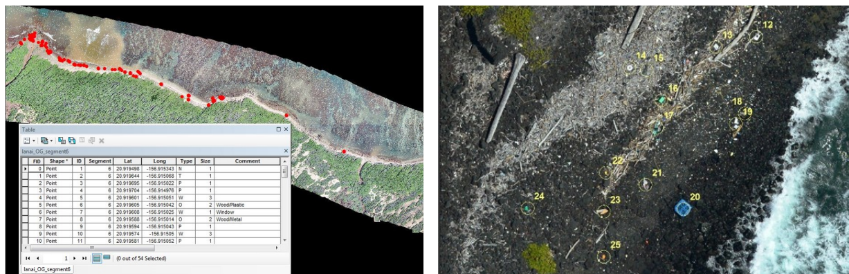
Figure 1: A swath of Kaua'i coastline in ArcGIS and the data table of the identified dots of debris (left), with a zoomed screenshot of identified marine debris with numbers on Kamilo Point, Hawaii Island (right)
