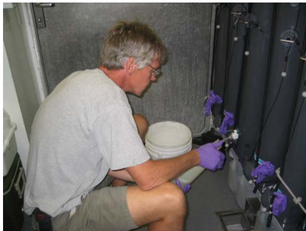
Fig. 12 Collecting filtered water from the Go-Flos in the University of Hawaii clean van. The 12 bottles are racked on either side of the van and filtration is accomplished through clean-air pressure
