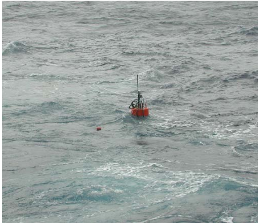
Fig. 14 The drifter, deployed. The small red float nearby is at the end of a tag line.
